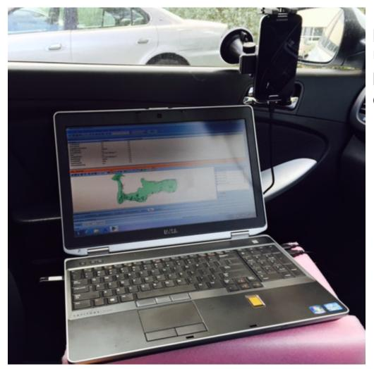
Drive Test Tool: Nemo Outdoor 7.1.1.12 User Equipment : Samsung S4 Model:SHG-I227 UD GPS: Garmin
